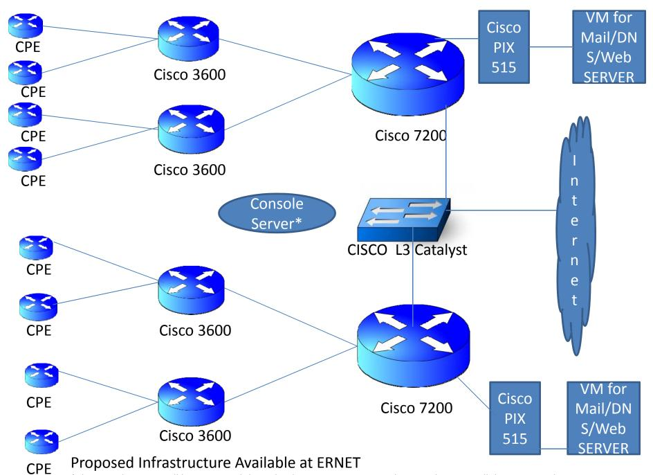
\*The console server will be connected through Ethernet on internet and on serial ports to all devices console ports. Training locations will access the central infrastructure over either ERNET network/ NKN or over the Internet.
